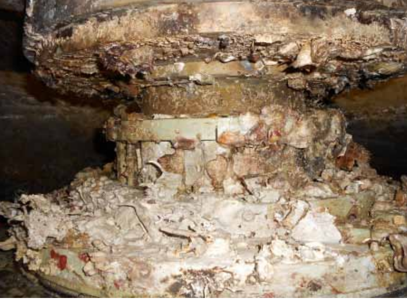
Thruster's propeller shaft seal after 1 year stand still.
