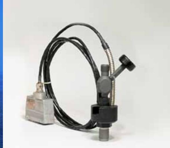
The unique cylinder pressure transducer is an integral part of the Intelligent Combustion Monitoring system which provides maintenance-free operation under MTBF of more than 10 years.
