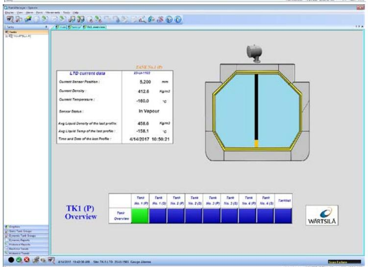
The gauges can be either connected to the Automation System through redundant RS-485 links, or to the Wärtsilä Whessoe Tank Data Acquisition system which includes Operation and Maintenance features.
