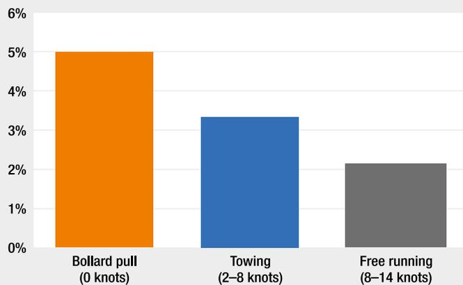
Performance improvement with the HP nozzle compared to 19A nozzle for a typical 150 ton AHTS.
