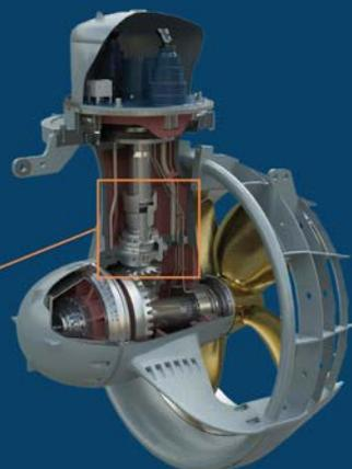
The spiral bevel gear-set, which is the heart of the thruster, has been thoroughly reviewed. Not only has the 8° gear angle been included in the gear geometry, the gear application and safety factors have been increased and a high quality gear material has been selected.
