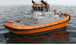
The Middle East's very first LNG fuelled tug, currently under construction at Drydocks World, Dubai.
