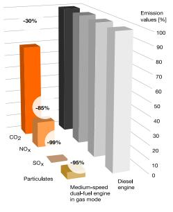
Example of emission reductions obtained by switching to gas.
