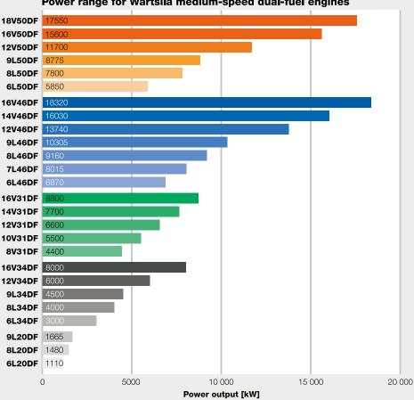
Wärtsilä's medium-speed dual-fuel engine portfolio for both main and auxiliary power production. The portfolio is available both for electrical and mechanical propulsion applications.
