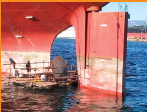
Trailing edge adjustment at pier side.
