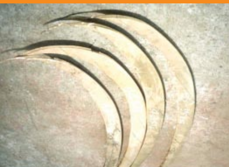
Equal pieces of propeller material are cut off.
