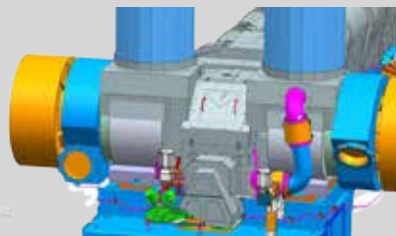
Integrated insulation box and turbocharger end insulation
